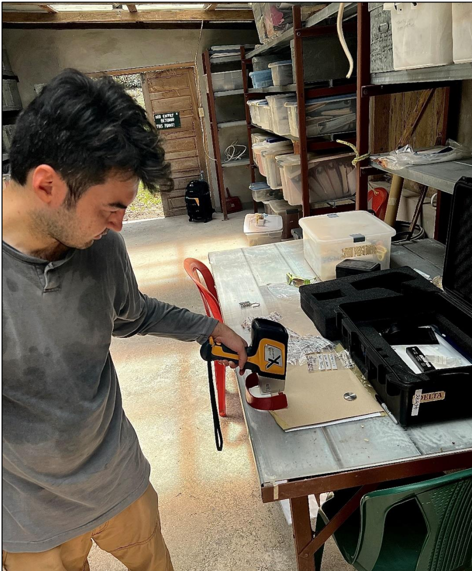
Photo shows Mike conducting pXRF (portable, non-destructive XRF) on ceramic samples in the lab
