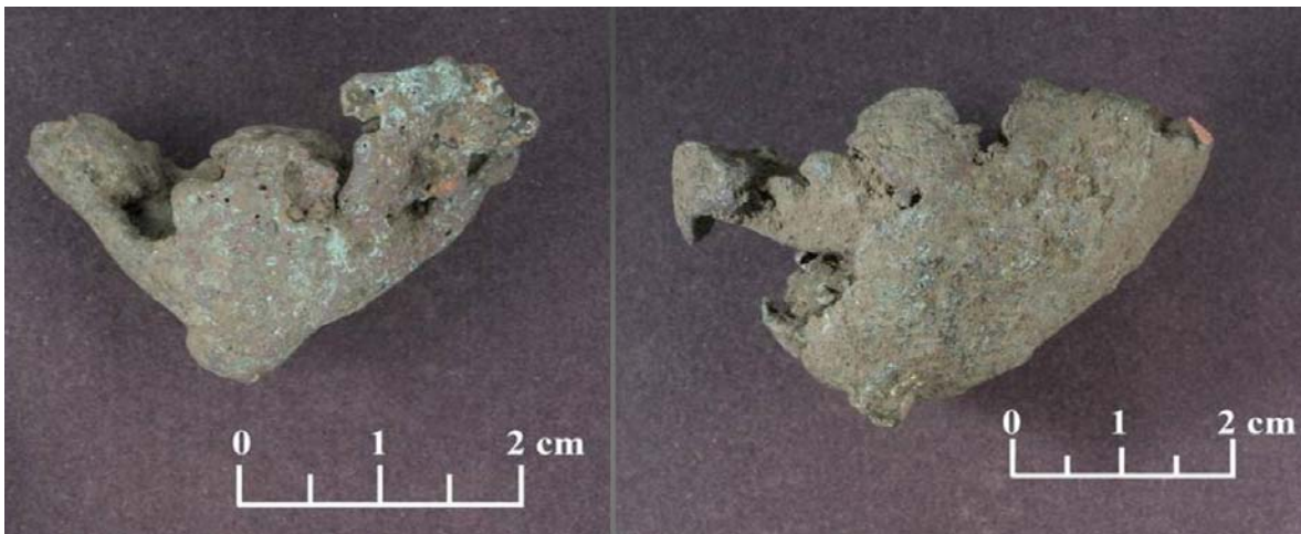
Figure 15: LA 2790-1 and LA 2790-4. These two previously termed ‘ingots’ are more likely pouring reservoirs from lost wax castings. Photo courtesy of Dan Kushel.
